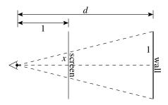
Because the triangles are similar, x/1 must equal 1/d. Thus the length of the wall's image as projected onto the screen is 2x = 2/d.
