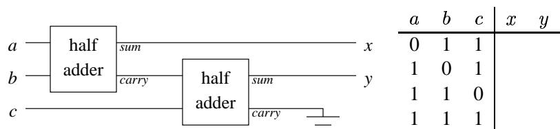
**Question 4.1–3:** (Solution, p S18) What distinguishes the behavior of a half adder from that of a full-adder? (That is, are their inputs or outputs different? Is the relationship between inputs and outputs different?)
