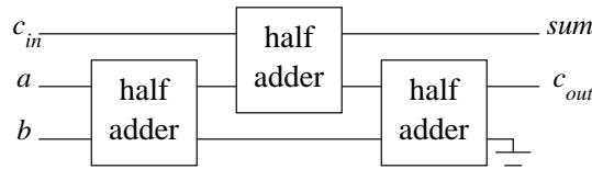
**Solution 4.1-6:** (Question, p S4) The design of this circuit is similar in structure to the design of a full adder using half adders.
